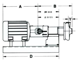
Note: Dimensions  $\mathbf{X}$ ,  $\mathbf{Y}$  &  $\mathbf{B}$  apply to pumps with clamp connection.
