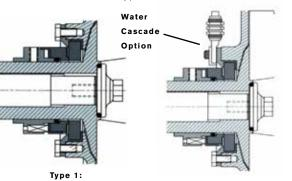
External Balanced Seal with Replaceable Mating Surface
